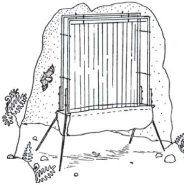
Fig. 3. Schematic representation of a harp trap set up at a cave entrance.
