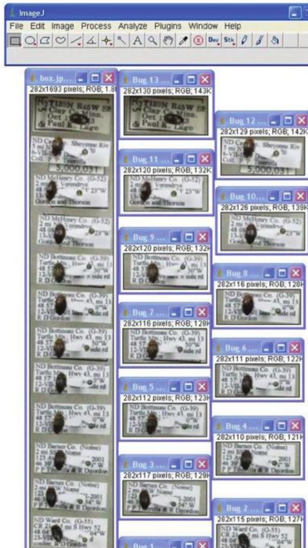
Figure 4. Image of multiple pinned insect specimens in unit tray (left) and same specimens segmented into separate files (right) using customized ImageJ image processing protocol.
