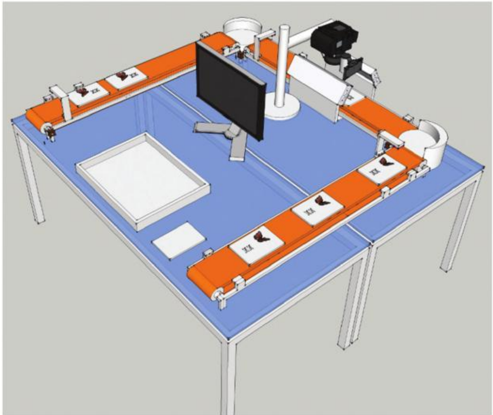
Figure 4. Conceptual design for automated imaging of entomological collections, which is currently being implemented at Digitarium.
