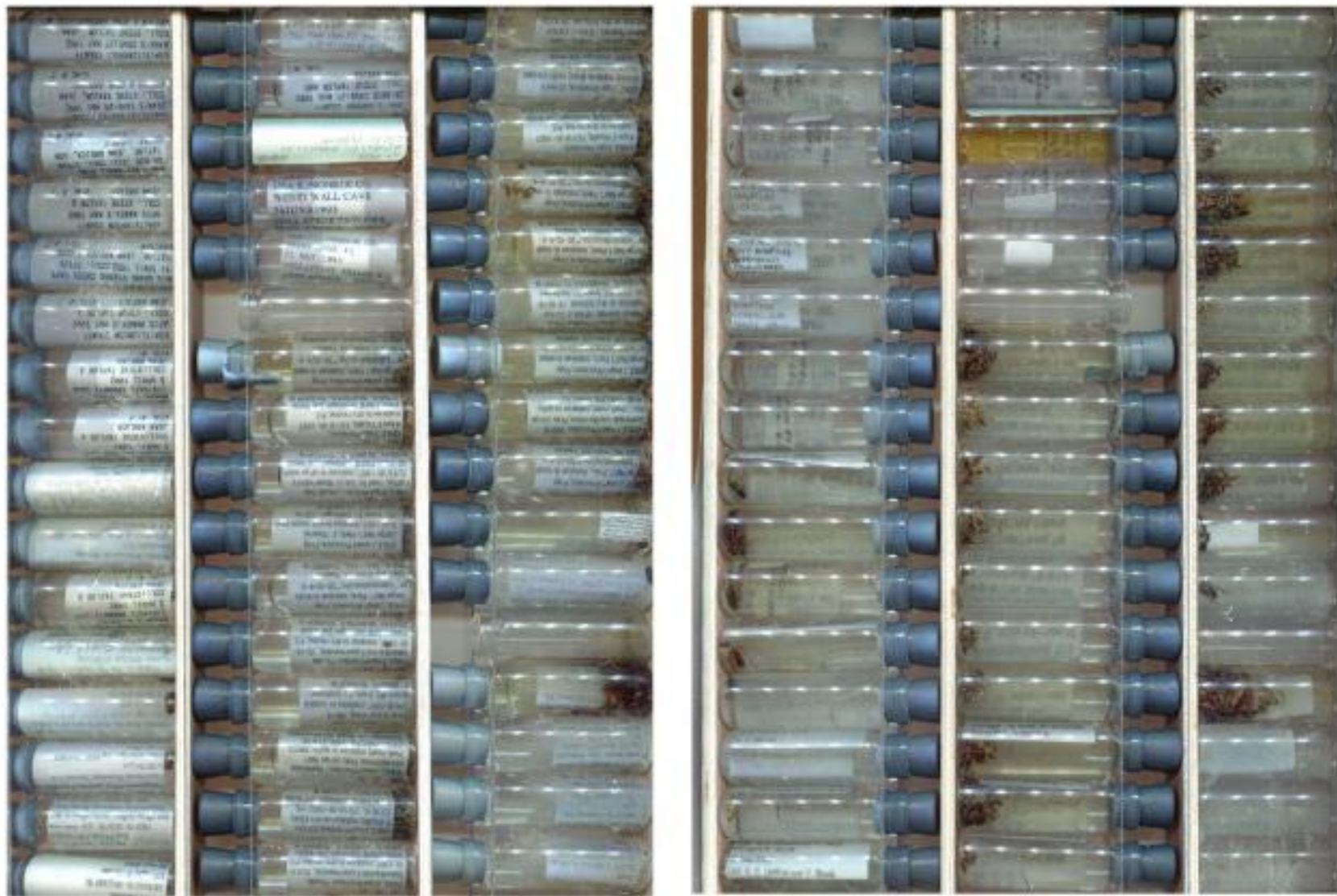
Figure 1. A set of three-dram vials scanned using a color flatbed scanner showing the front (left) and back (right) of the same set of vials. Note that the position of empty spacer vials (e.g., sixth from top in middle column) is the same, but inverted, in the two images because the vial racks are flipped vertically between scans. This relatively quick and inexpensive procedure exposes at least some label data for subsequent capture and reveals the general condition of specimens.
