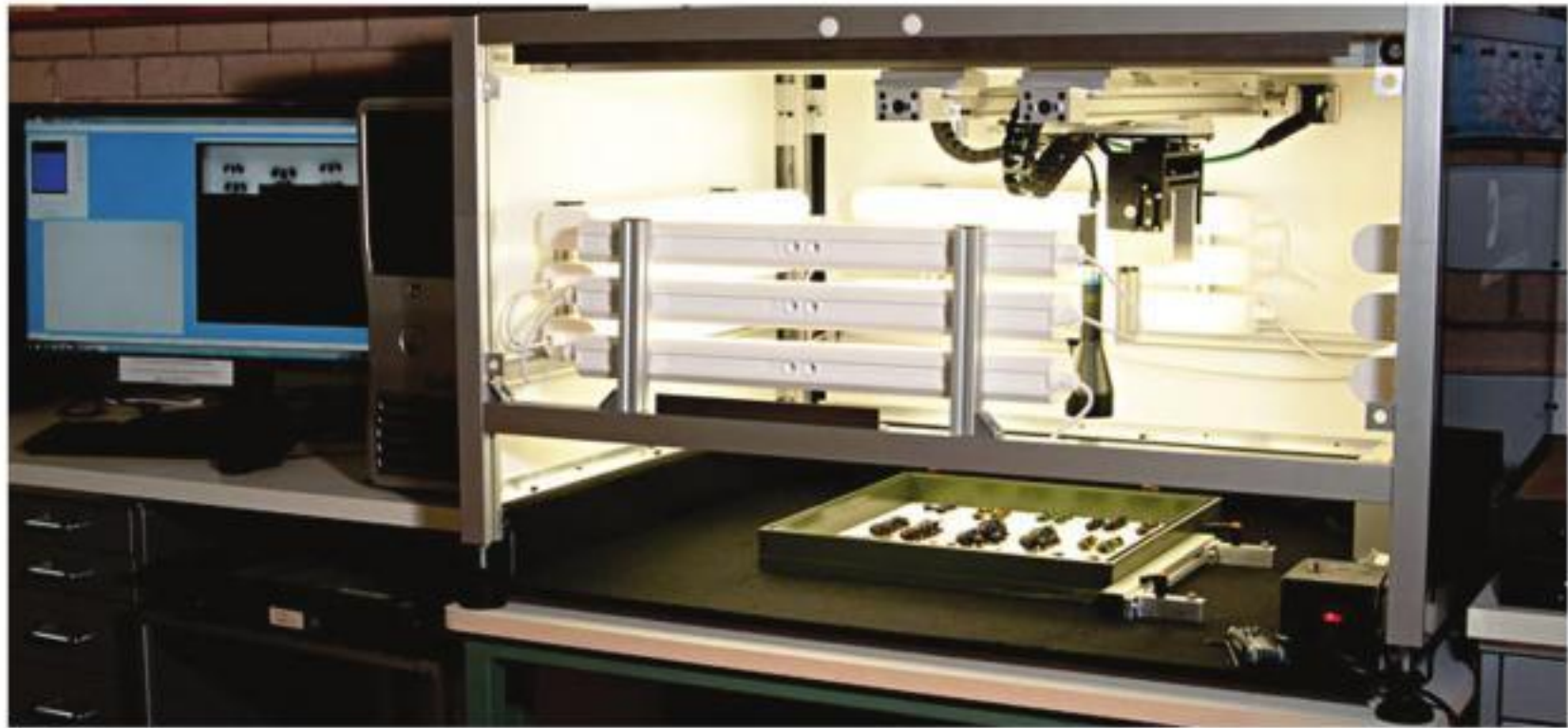
Figure 1. The SatScan imaging system used in ANIC. Shown here with the front cover removed.
