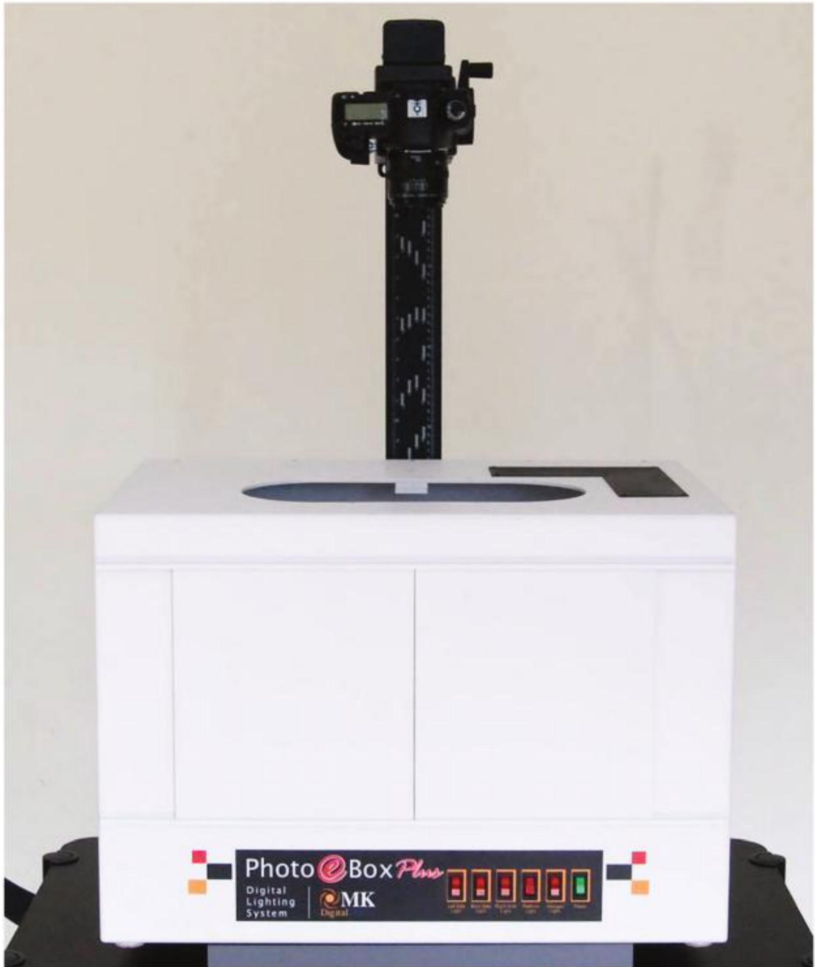
Figure 2. NYBG imaging station consisting of a Canon Eos 5D Mark II digital camera body, a Canon EF 50mm f /2.5 Macro lens, Photo e-Box Plus 1419 from MK Direct, and Kaiser RS 1 copystand.
