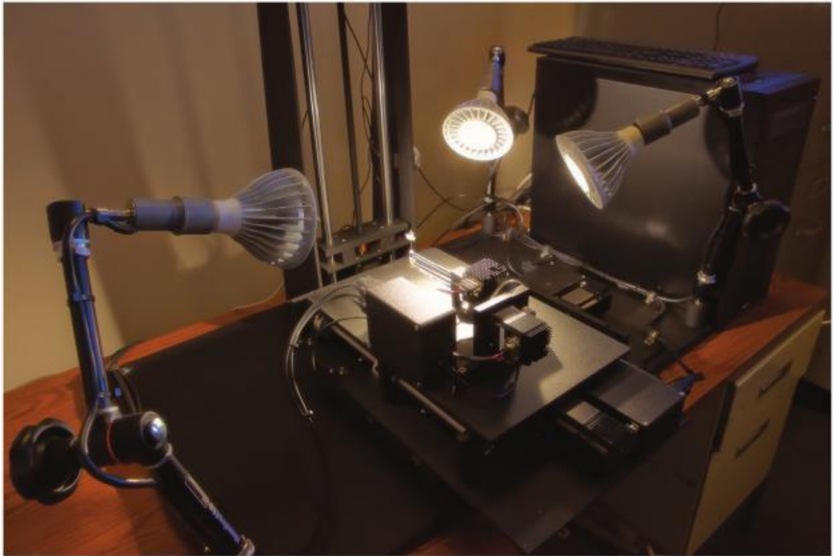
Figure 2. Two ROBOT(E) remotely operable digital imaging systems designed to allow taxonomists to examine, manipulate, and digitally photograph type specimens through a Web connection. Three such instruments are being deployed to major insect collections in Washington, London, and Paris. A prototype instrument remains with the IISE for testing and development purposes. PHOTO: Courtesy of Erik Holsinger, Arizona State University.
