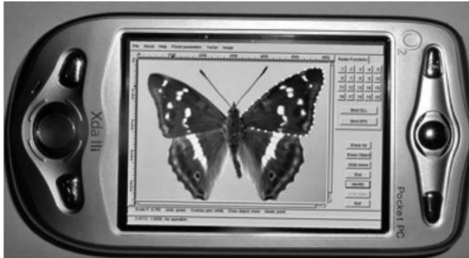
FIGURE 7.15 DAISY running on the PocketWindows desktop under pocket Tux-Linux parasite on an Xda II i Pocket PC.
